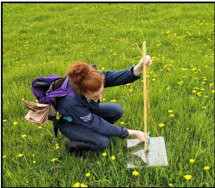
Using a homemade falling plate meter. Image from www.fieldcropnews.com .
